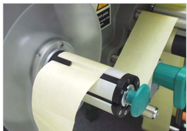
[44] Fastening the backing paper to the rewinder.
