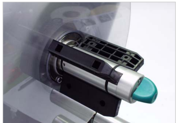
[46] Core adapter positions for a core diameter of 101.6 mm.
