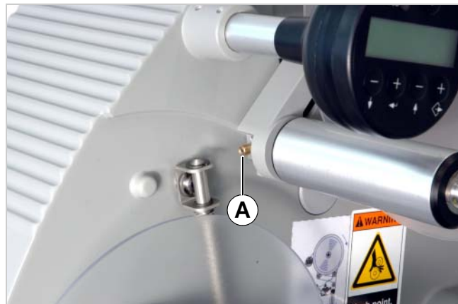
[49] Setting screw (A) at the unwinder dancer arm.
